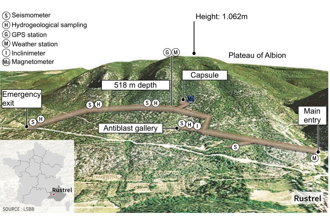
The LSBB counts with 54ha of surface and 4 km of underground galleries with depths ranging from 0 to 518 m
