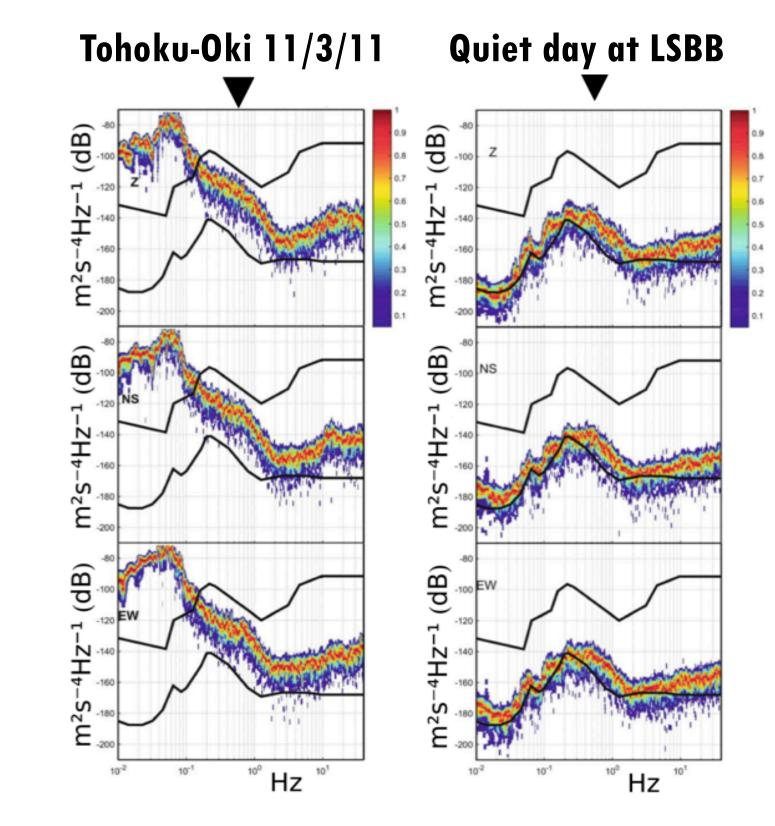
PSD (top to bottom: Z, NS, EW) vs Peterson's high and low noise models
